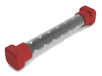
These marbles are used as digestion enhancers and to prevent the pancreas from moving in unison with the chamber. The marbles enhance the dispersion of pancreatic tissue inside the chamber. Diameter: 5/8" (15.875 mm).
